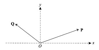
Two horizontal forces  $\mathbf{P}$  and  $\mathbf{Q}$  act at the origin O of rectangular coordinates Oxy (see diagram). The components of  $\mathbf{P}$  in the x- and y-directions are 14 N and 5 N respectively. The components of  $\mathbf{Q}$  in the x- and y-directions are -9 N and 7 N respectively.
